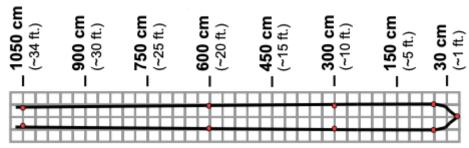
Typical beam patter for 30cm target mover left and right with the board parallel to the sensor face
